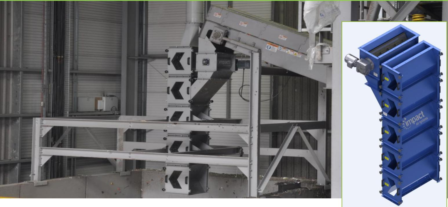
The Impact zigzag system is a fully adjustable cascade cleaning solution, suitable for most types of free flowing material streams up to 60mm in size to remove unwanted low density material.
